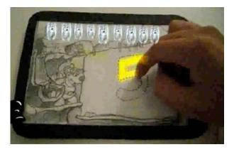
Figure 8: Example of usability testing with a low-fidelity executable prototype
