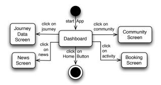
Figure 6: UML state diagram representing the user interface modeled in figure 5
